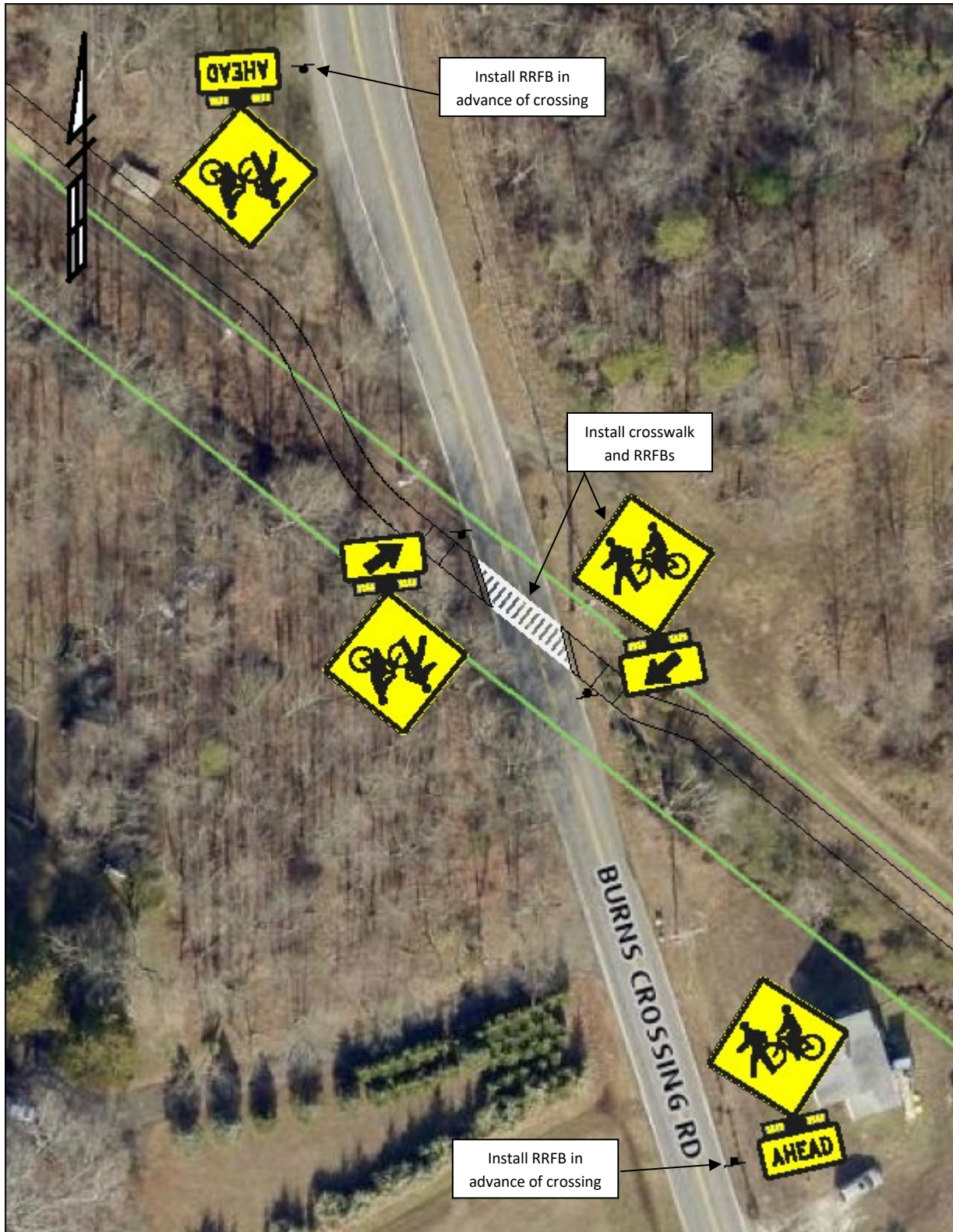
Figure 1: Burns Crossing Road Recommended Improvements
