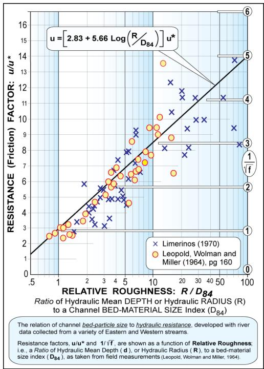
Figure 2-18. Relative roughness (R/D<sub>84</sub>) vs. friction factor (u//u\*).
