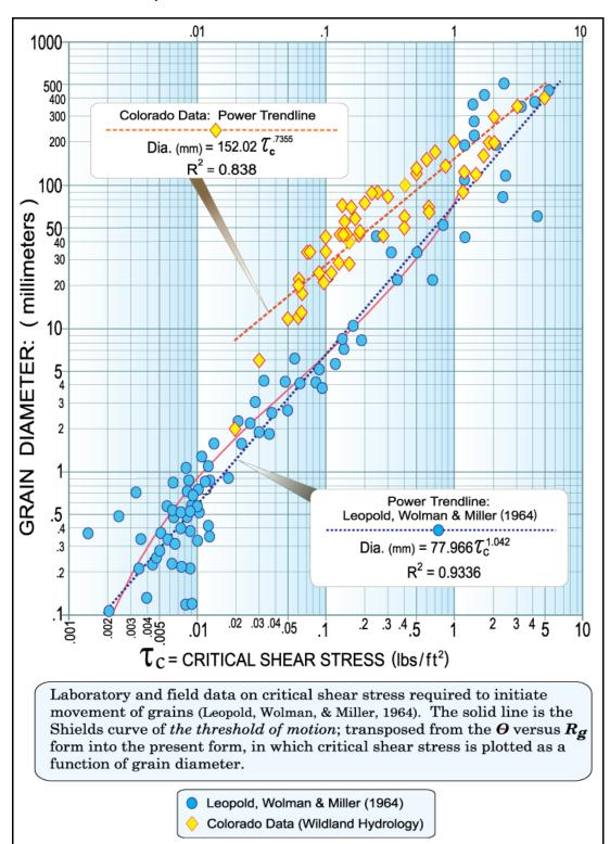
**Figure 3-11.** Critical shear stress required to initiate movement of bed-material grains following the Shields relation, as modified by field data from Colorado.
