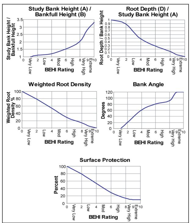
**Figure 3-7.** Streambank erodibility criteria showing conversion of measured ratios and bank variables to a BEHI rating. Use **Worksheet 3-11** variables to determine BEHI score.
