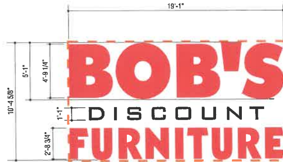
1 STACKED CHANNEL LETTER LAYOUT 198.2 sf SCALE: 3/16" = 1' 0"
