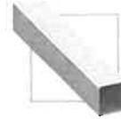
FRONT/BACK WALL GIRTS 1.5" Square 18 Gauge Galvanized Flush Mount Girts 3' 9 1/4" On Center Spacing
