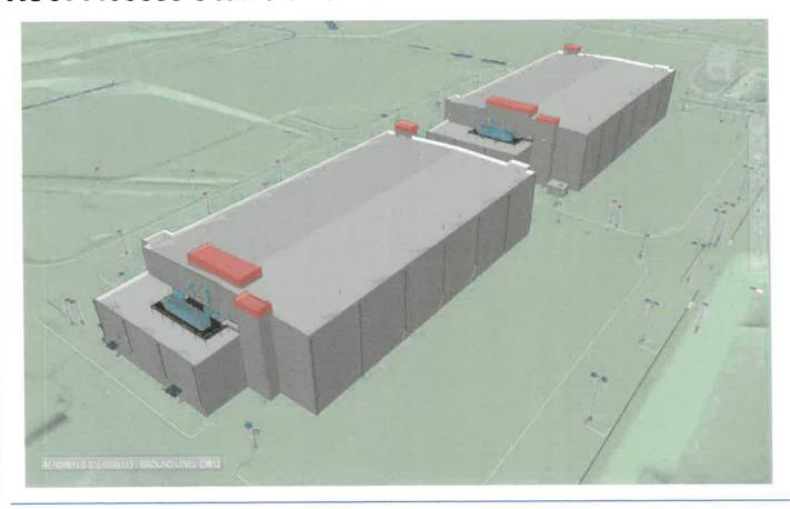
Two Roof Access Stairs, and the Elevator Machine Room Bulkhead comprise 2 ½ % of the overall building footprint. The upper 5'-0" of each are highlighted in red, as that portion of each exceeds the allowable building height defined in the Zoning Code.
