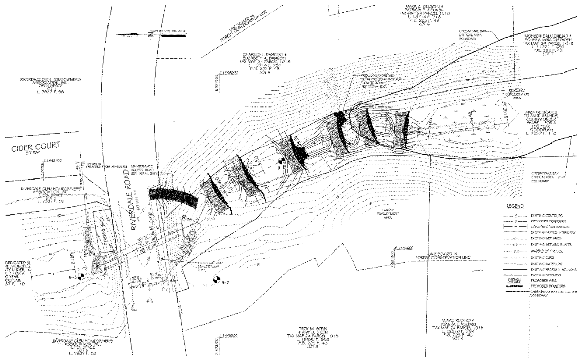
Figure 18: Example Retrofit of Eroded Outfall – Post-Reconstruction Severn Run Outfall Repair
