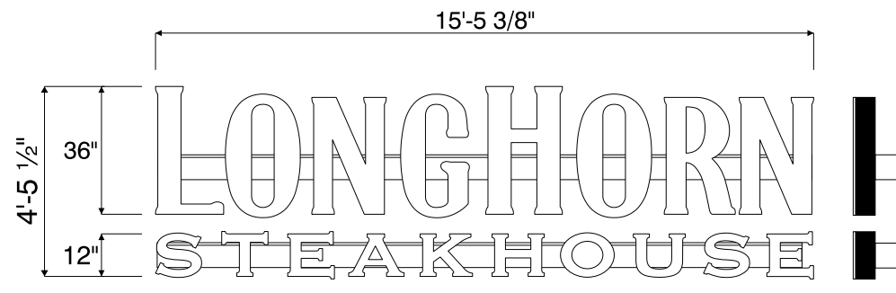
D 36" Channel Letters on Raceway (Internally Illuminated w/LED) Utilized Square Footage: 68.9 Scale: 1/4" = 1'
