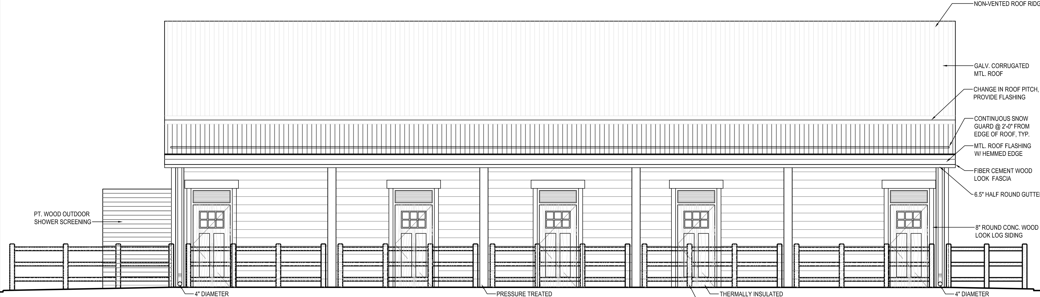
1 BATHHOUSE WEST ELEVATION SCALE: 1/4"=1'-0"
