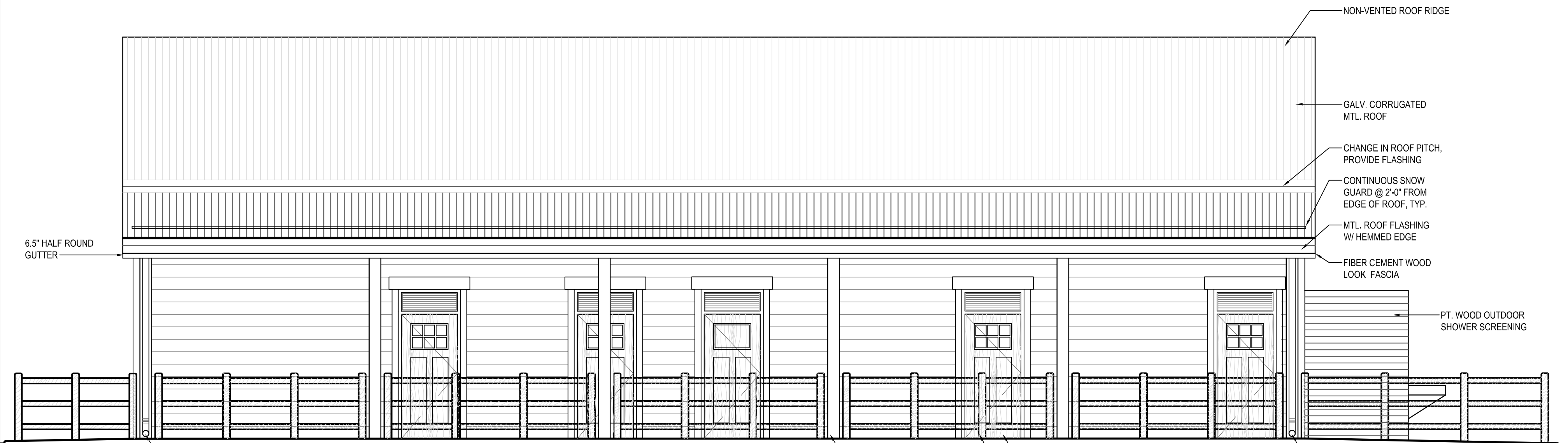
1 BATHHOUSE EAST ELEVATION SCALE: 1/4"=1'-0"
