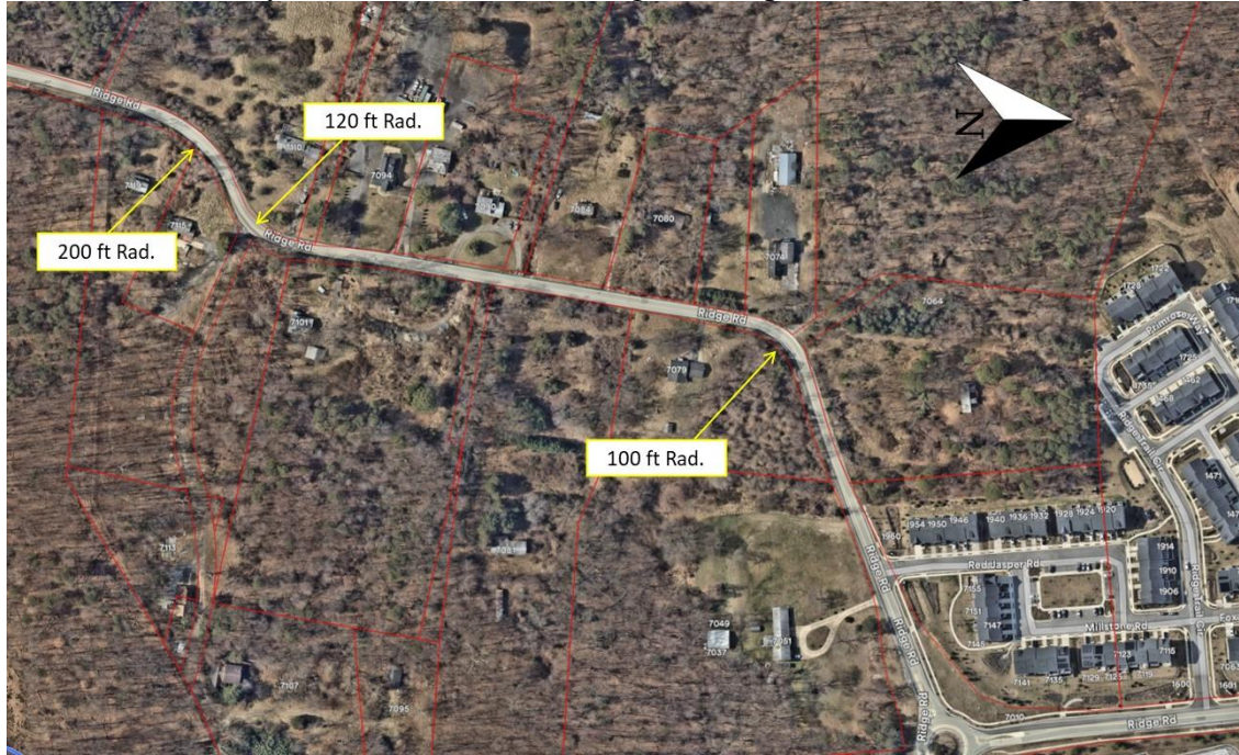
Figure 14: Substandard horizontal curvature, south of The Ridge development
