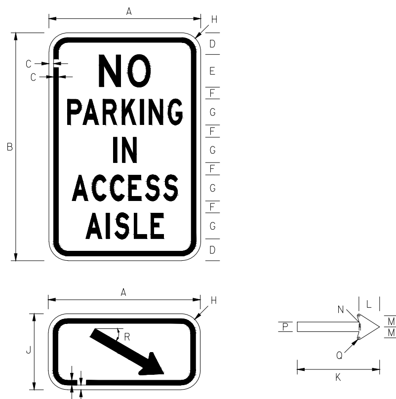
ACCESS AISLE SIGN DETAIL NOT TO SCALE
