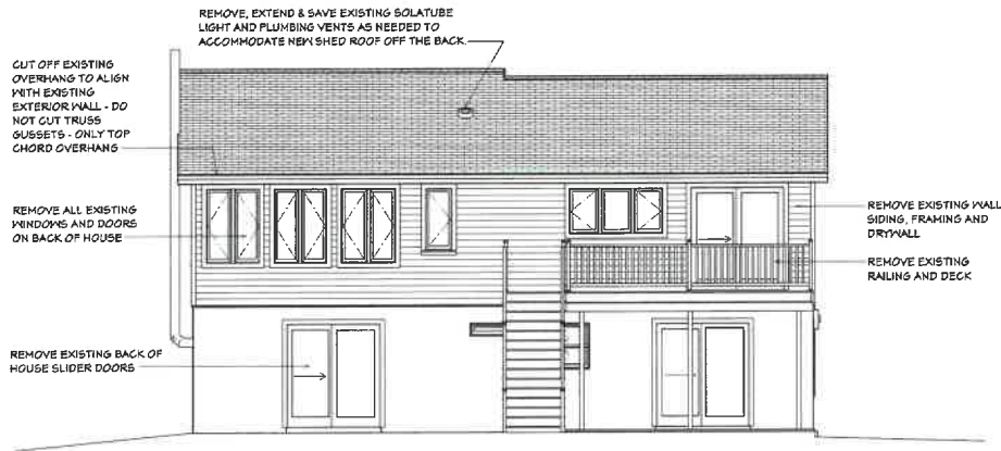
AS-BUILT/DEMO NORTH ELEVATION 1/4" = 1'-0"
